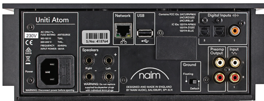
The rear of the Atom has both digital and analogue inputs - although the latter is routed through an ADC (see Measured Performance for further details).
