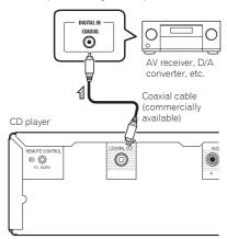
The audio of iPod/iPhone/iPad mini is not output from the COAXIAL OUT socket of the CD player.
