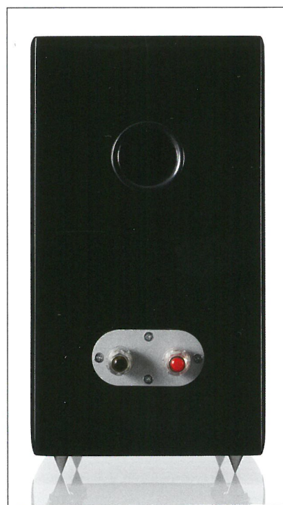
The bass reflex port is located on the rear of the speaker, and can be damped if necessary. The bottom of the cabinet features recessed threaded sockets to take spikes or glides.
