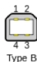
This is a USB-B port. This is the connection we will explain in this document in more details.
